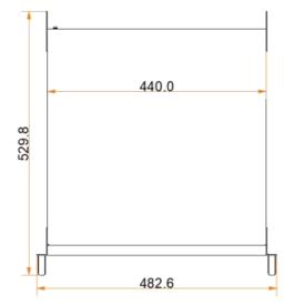
Tolerance: ±0.3 Unit: mm
