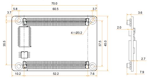
Tolerance: ±0.1 Unit: mm
