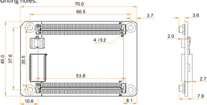
Tolerance: ±0.1 Unit: mm
